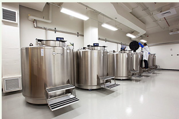
Nitrogen freezers housed in the National Museum of Natural History's Biorepository. These freezers, along with others across the Global Genome Initiative, will be used to cryo-preserve 50% of the diversity of life in five years. Credit: Donald E. Hurlbert, Smithsonian Institution
